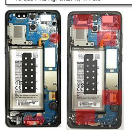
Assemble Front assy on REAR vertically.
