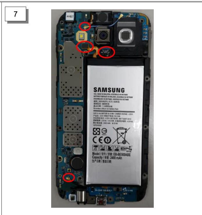
1) Detach Connector and Coaxial Cable from PBA
