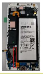
Assemble the Main PBA to Bracket and connect the 4 connectors well.
