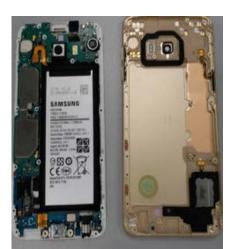
6 Disassemble the coaxial line from PBA
