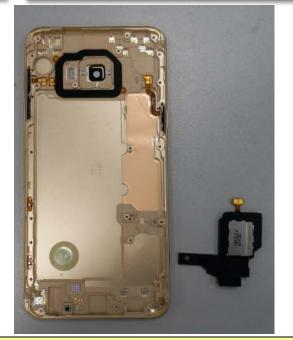
Assemble Bracket Assay and Rear Assay and Assemble 21 screw into Rear.
