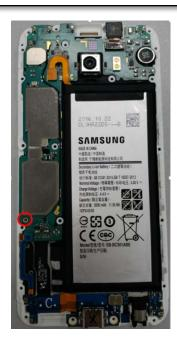
8 Assemble the 2 coaxial line to Main PBA.
