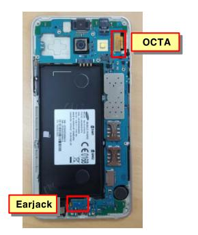
6 Disassemble the PBA.
