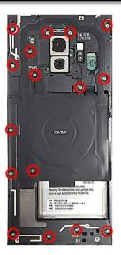
Attach the finger sensor on the REAR and Assemble the finger sensor on the PBA
