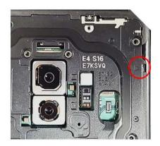
Rear Top disassemble hole.
