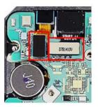
Attach 2 coaxial cable, Battery connect and the other connectors. (8 Point)
