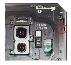
Rear Top disassemble hole.
