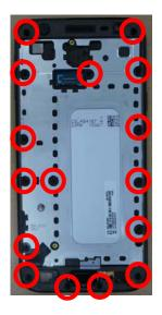
Replace all non-reusable tapes to the new one, and assemble LCD connector and connector cover and Attach LCD
