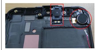
6 Assemble the PBA and connect FPCB.
