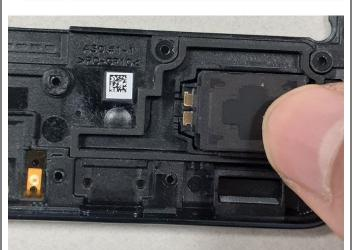
2 Attach screw and Sub PBA on Front Ass'y.
