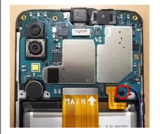
Remove the PBA and C to C FPCB and Batt Conn and BLACK, Blue coaxial cable and VT
