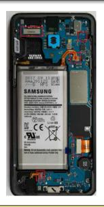
6 Disassemble PBA from Front. (like ①② image)
